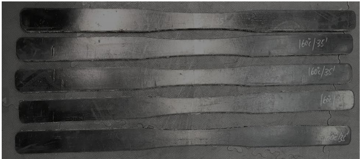
Figure 32. Conveyor belt specimens for tensile test prepared from samples vulcanized at 160 °C for 35 minutes.
