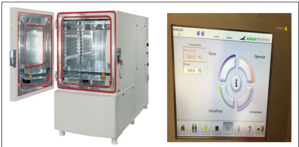
Figure 20. (a) Industrial temperature chamber (Industrial oven), (b) Temperature monitoring part of the oven.
