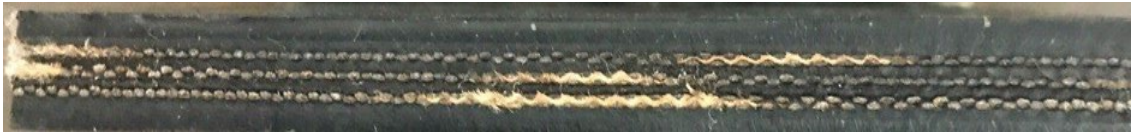
Figure 25. Side view of EP fabric reinforced conveyor belt with three-layers and produced with the vulcanization parameters of 160 °C for 35 min.
