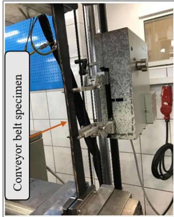
Figure 33. Conveyor belt specimen under tensile load.
