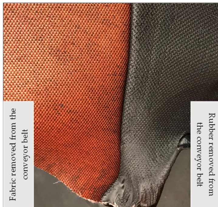
Figure 58. Woven fabric sample manually removed from sample vulcanized at 140 °C for 6min.
