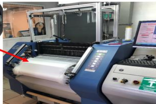
Figure 8. Loom preparation and fabric manufacturing process, yarn winding on weaver's beam, drafting, denting, and weaving process.
