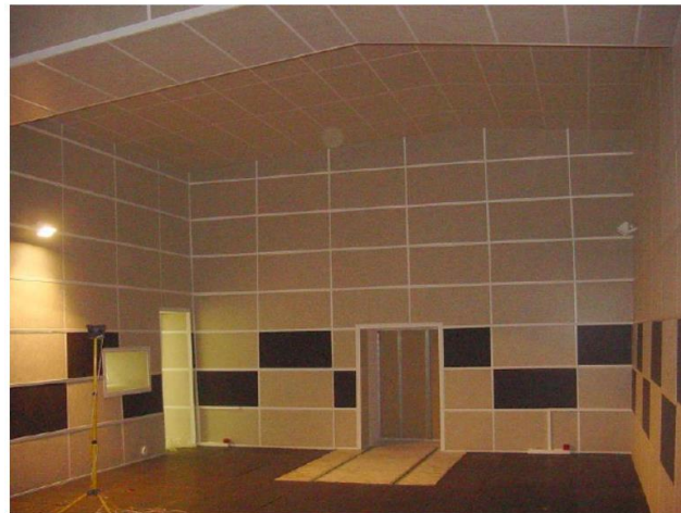
Figure 4. Aeroacoustics chamber at Łódź University of Technology Institute of Turbomachinery [83]. Contains 368 m 2 of aeroacoustics room dimensions surface area.
