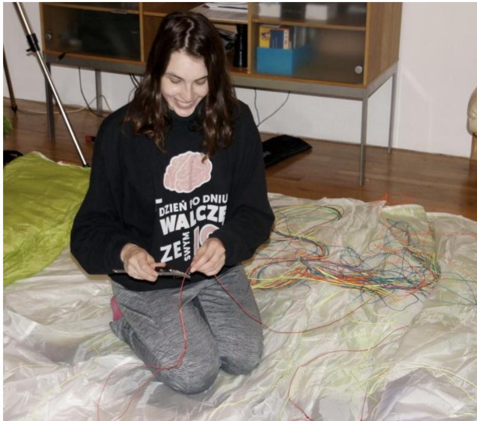
Figure 58. measuring the diameters of the lines of the considered paraglider
