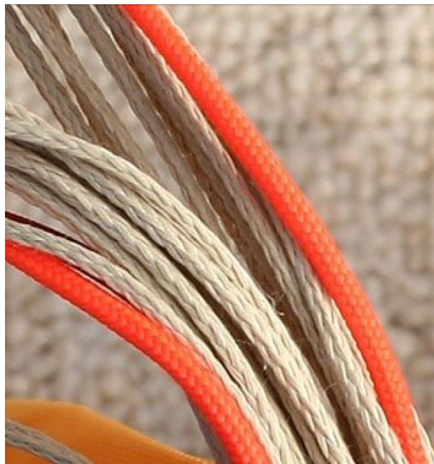
Figure 56. Aramid braided core of paraglider lines (lines without outer sheath) and the same type of paraglider lines with the outer PET sheath (orange) [6]
