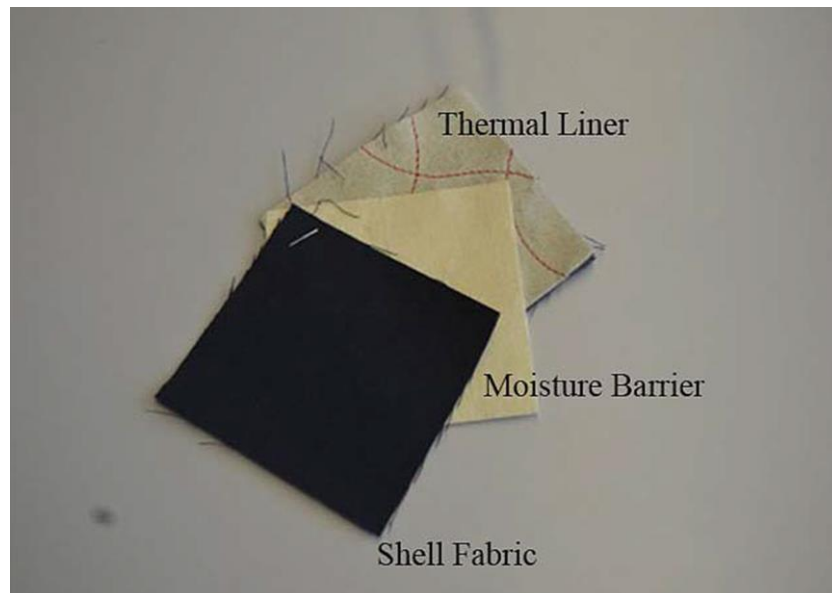
Fig. 2.8. Exemplary picture of layers applied in the FPC [33]
