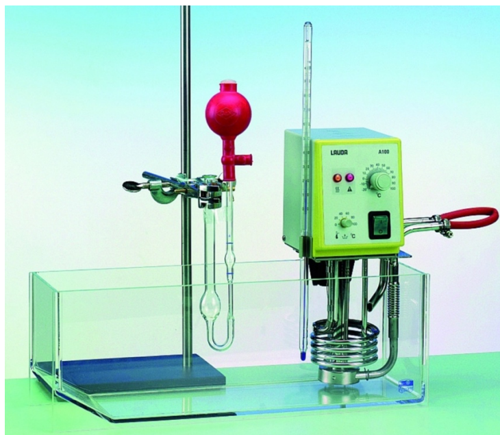
Rysunek 18. Stanowisko do pomiaru lepkości roztworu polimeru (Determining the Molecular Weight of a Polymer from Intrinsic Viscosity Measurements | PHYWE, n.d.)
