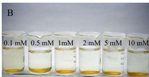
Figure 13. Photographs of 0.1–10 mM FAS solutions after preparation (0 h) (A) and storage for 24 h (B), 72 h (C), 168 h (D) in a refrigerator ( \sim 4^{\circ}\text{C} ) for the solutions prepared in distilled water.
