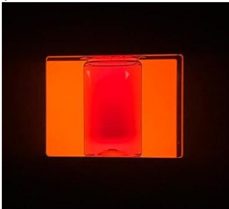
Figure 11. Fricke-XO-Pluronic F-127 dosimeter irradiated according to the calibration plan ( Figure 10B ) placed in OCT with orange light (589 nm) turned on. Sample seen from the CCD (Charged-Coupled Device) matrix side of the tomograph.
