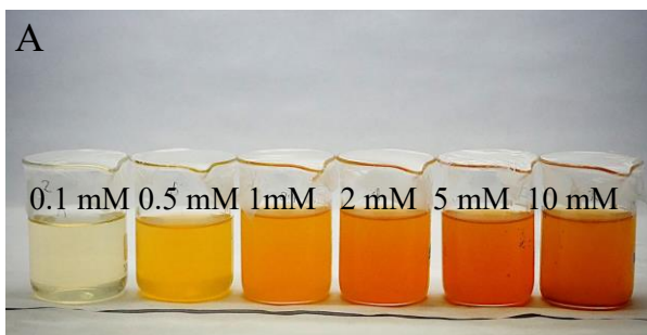
Figure 11. Photographs of 0.1–10 mM FAS solutions after preparation (0 h) (A) and storage for 24 h (B) and 48 h (C) in a refrigerator ( \sim 4^{\circ}\text{C} ) for the solutions prepared in tap water.
