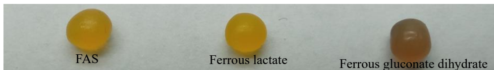
Figure 30 Examination of diffusion of Fe (A, C, F) and Ca (B, D, G) from alginate capsules (average weight of one capsule: 0.034 g) made by reaction of sodium alginate solution (Sigma) (3.5%) with Fricke solution (FAS: 1 mM, H 2 SO 4 : 50 mM, XO: 0.165 mM; reaction time= 40 min) containing 3.5 CaCl 2 (A, B), different concentrations of FAS (C, D), and different compounds containing Fe (F, G) (concentration of each compound: 1 mM). In E and H, the photographs of capsules made of different concentrations of FAS and different compounds containing Fe, respectively, are shown. The capsules were immersed in 3.5 mL of re-distilled water. Measurements performed with the aid of ICP-OES. For A and B, the water with the capsules was changed after 48 hours of diffusion, for C and D, the water was changed after 180 minutes, and for F and G, after 120 minutes.
